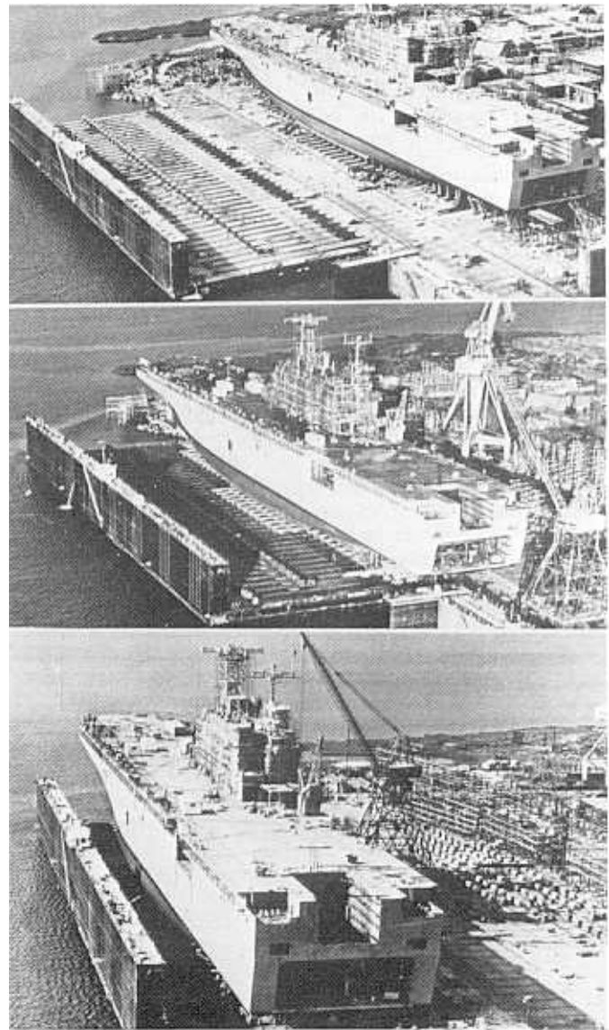
Fig. 5 Three stages of LHA transfer photographed at Litton's Pascagoula yard using 57,000-ton floating dry dock with side transfer capability
